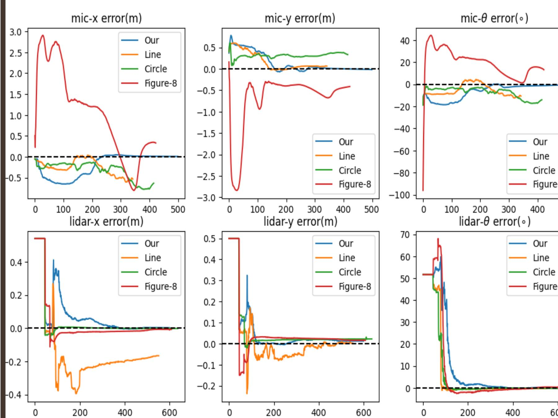
Microphone array and LIDAR external parameter estimation errors
